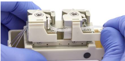
Figure 16: OFM Tubing Set is fixed with retaining springs in the pump.
